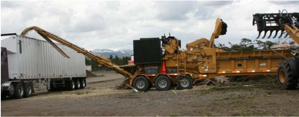
Figure 4. Machine chips forestry waste and deposits into chip van for transport (Searcy, 2010)
