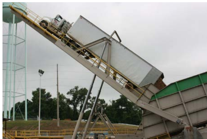
Figure 5. Chip van is unloaded into conveyor system for processing at plant (Searcy, 2010)
