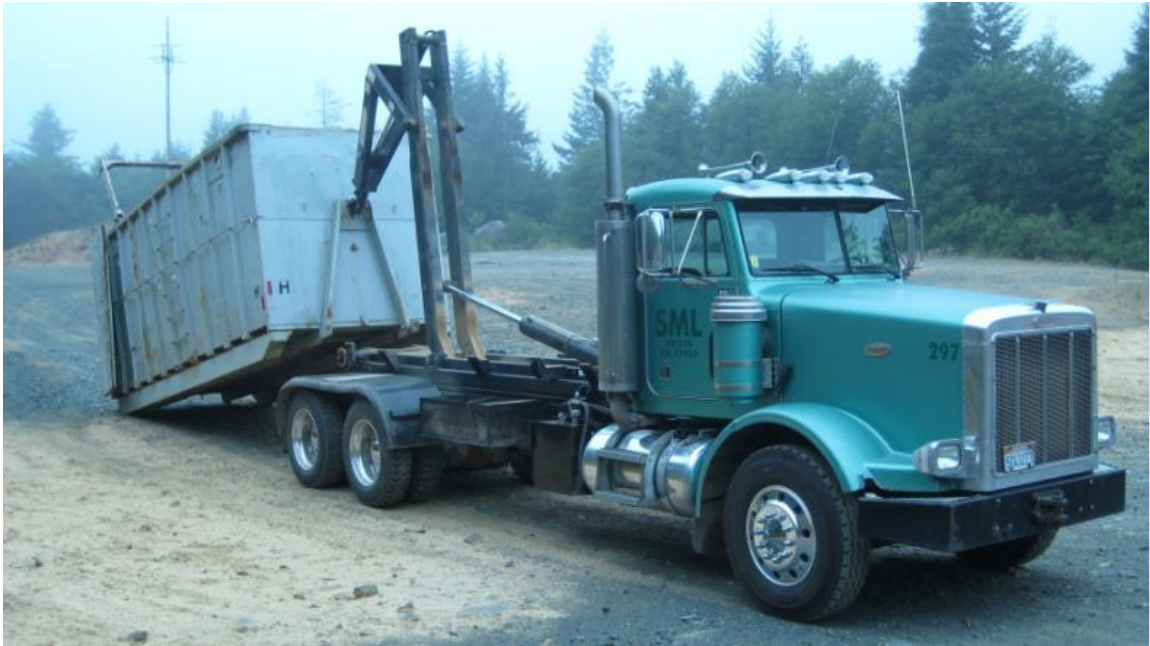
Figure 1. Hook-lift truck with 40 cubic yard bin used to transport forest residues to centralized grinding site.
