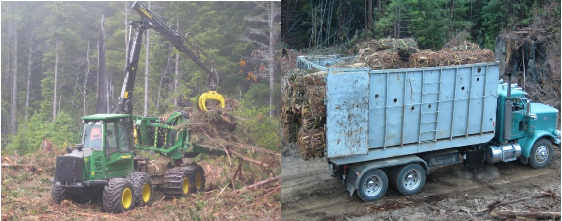
Figure 6. John Deere 1490D energy wood harvester which produces the bundles, and hook-lift truck used to haul bundles.
